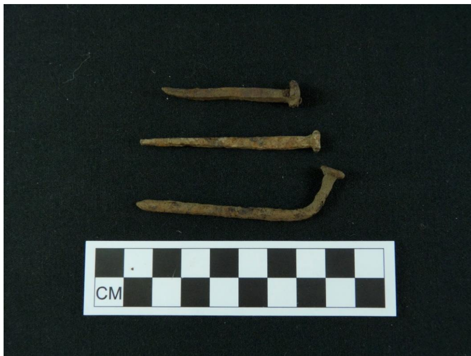
Image 14: (Top to bottom) wrought nail (920E 955N: 25), machine cut nail (925E 950N: 01), and wire nail (910E 940N: 08).
